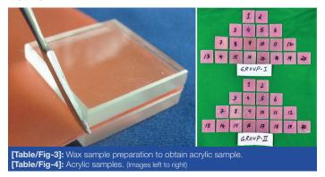
The advancing and receding contact angles of saliva substitutes were measured on acrylic samples using contact angle goniometer [14] (DSA25, KRÜSS) and software (DSA4) [Table/Fig-5] by following method: a pre-sterilized glass syringe was filled with measuring liquid (*Aloe vera*). Liquid drop was standardized with the help of graduated
