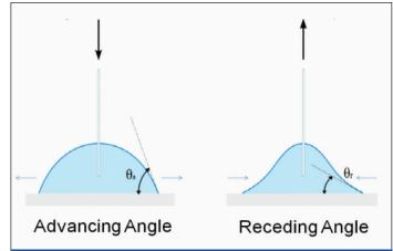
[Table/Fig-7]: Illustration of advancing and receding contact angles.
