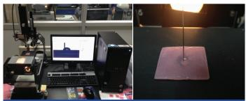
[Table/Fig-5]: Contact angle goniometer (DSA25, KRÜSS). [Table/Fig-6]: Measurement of contact angles using goniometer syringe. (Images left to right)
